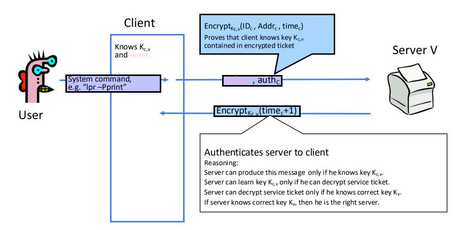
For each service request, client uses the short-term key for that service and the ticket he received from TGS
